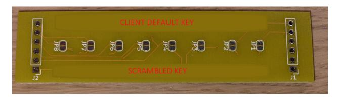
To make the addon work with your stations, first you must cut the default connection and then rewire the connection to match the scrambled key.
